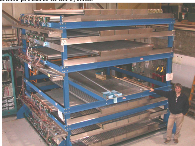
Fig. 1 The 20' tall Large Muon Tracker (taken October 2006), a sub-scale prototype built at Los Alamos National Laboratory, will vet the detector technology needed to field a full scale device. Overlapping X and Y detector planes are used to get the precise positions of the muon tracks above and below the sampling region. Also shown are the new redundant detector planes to improve tracking efficiency & quality.
